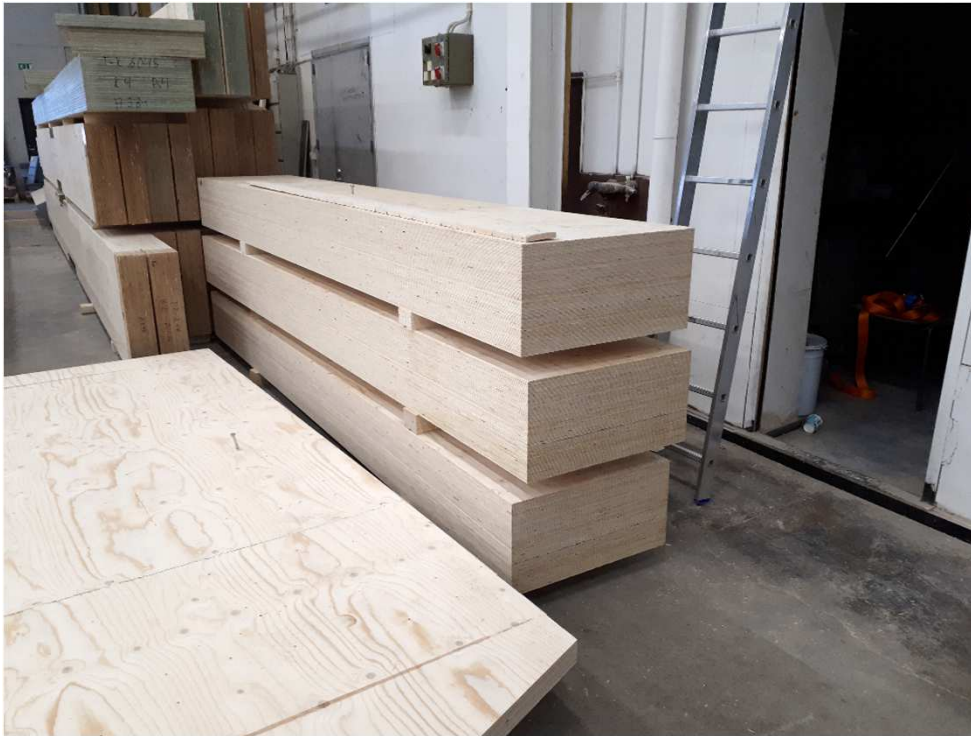
LVL G posts and beams, dimensions 225x600 & 225x450
