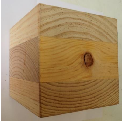
Fig. 2.18. Cross-laminated timber consists of orthogonally glued laminations. It is a versatile product that can be used as a slab or a wall, as seen here.
