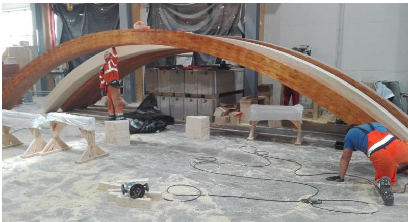
Fig. 7.3. Curved glue-laminated wood arches (Gadalabākābūve Latvijā 2017, 2018. The best building of the year in Latvia, 2018)
