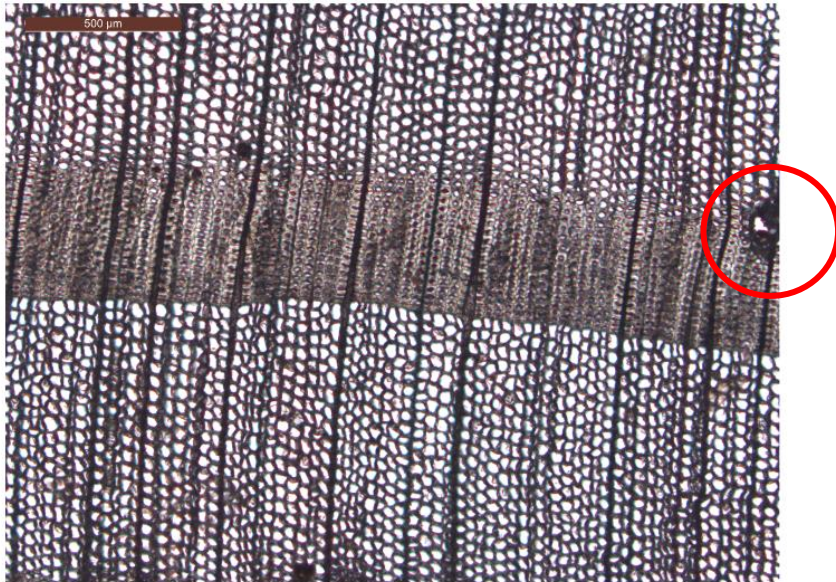
Fig. 2.8. Transverse section through a Scots pine. Morwenna Spear © Chris Miles.
