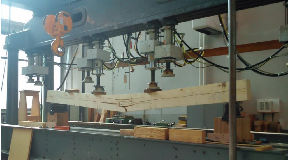
Fig. 2.14. Four-point bending test to a piece sawn softwood at the University of Stuttgart. © David Trujillo.
