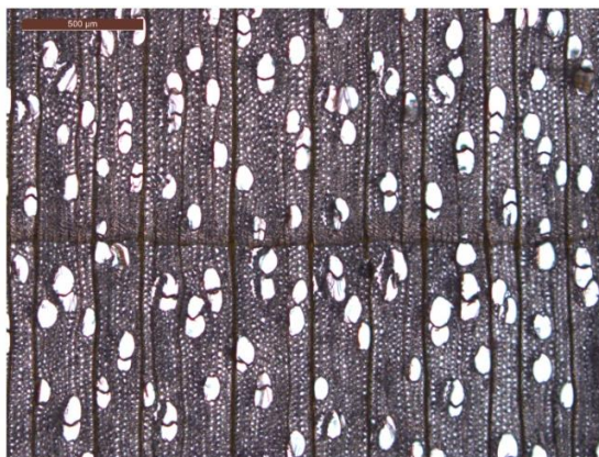
Fig. 2.10. Transverse section through birch. Morwenna Spear© Chris Miles.
