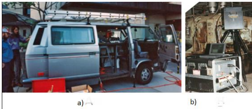
Fig. 6.2. Cyrax laser scanning system: a) prototype, b) model Alpha (Cheves, 2014).
