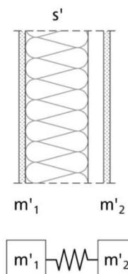
Figure 5: mass/spring/mass system (double layer wall) [2]
