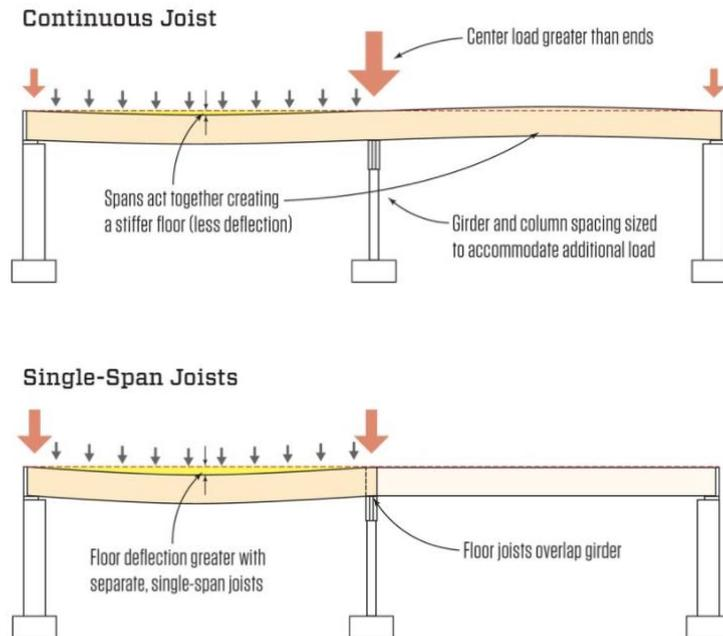
Figure 2: Comparison of single and multi span beams
