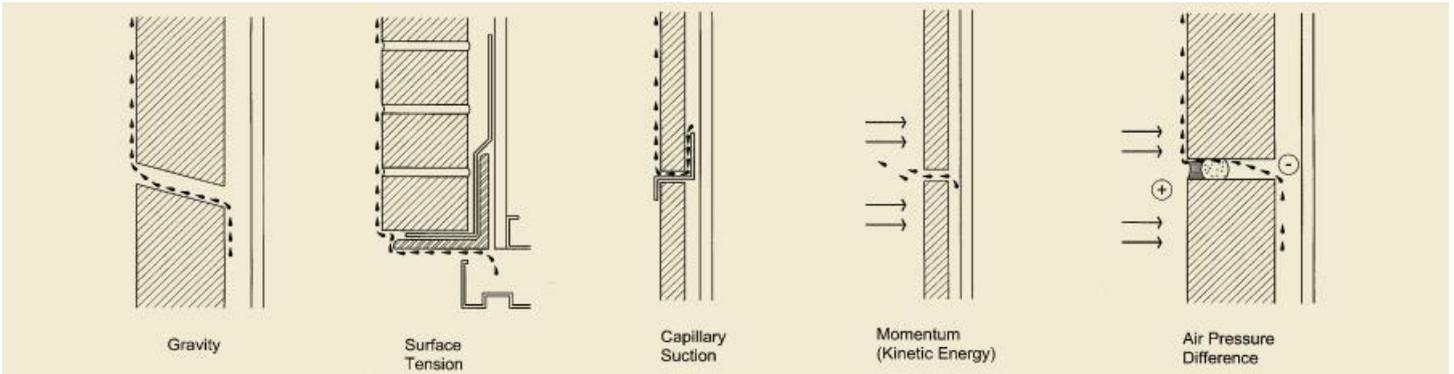
Figure 1: Driving forces that may be present in the construction
