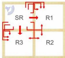
Figure 1: Transmission of airborne sounds via walls [1]
