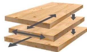
Figure 4: Cross-laminated timber [1]
