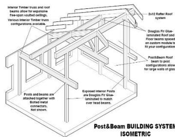
Figure 3: Post-and-beam construction [1]
