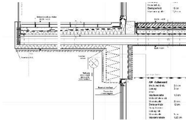
Figure 3. Example: Mitigation of thermal energy dissipation in cantilevered timber structures [6]
