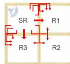
Figure 3: Transmission of airborne sounds via walls [3]
