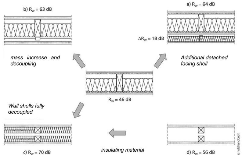
Figure 6: improvement measures for timber frame constructions[2]
