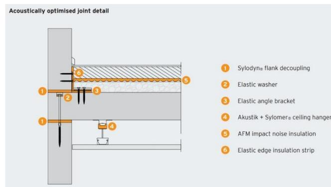
Figure 1: Separation joints
