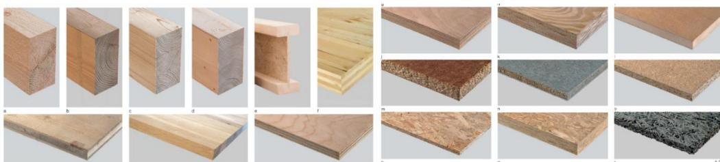
Figure 1: Common solid wood products and wood-based materials
