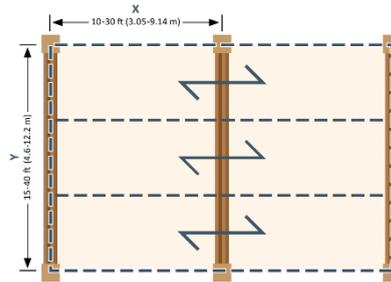
Figure 1: Typical post-beam-panel system grids
