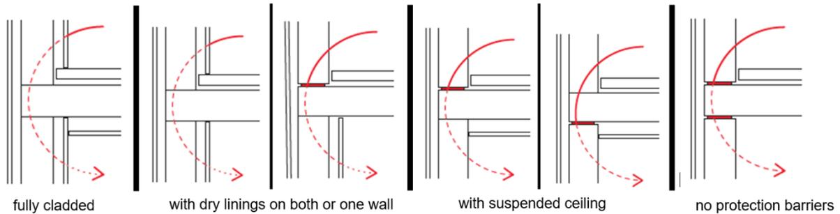
Figure 4: Basic construction rules for the need of elastic separation layers [3]
