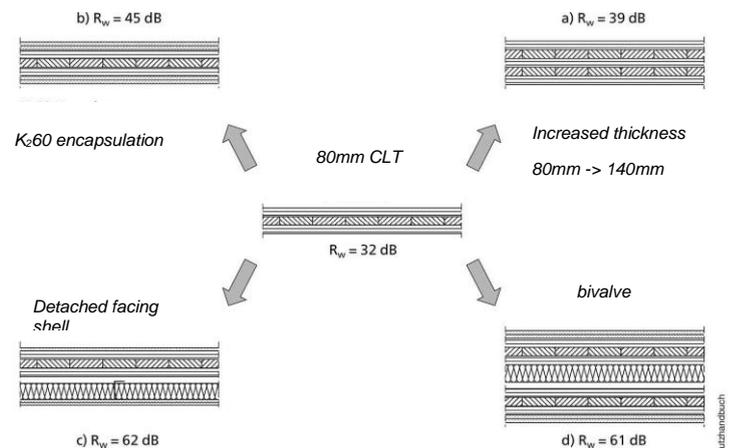
Figure 6: improvement measures for solid timber constructions [2]
