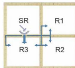
Figure 2: Transmissions of impact sounds in walls [1]
