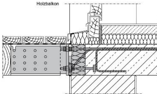
Figure 2. Example: Mitigation of thermal energy dissipation in cantilevered timber structures [6]
