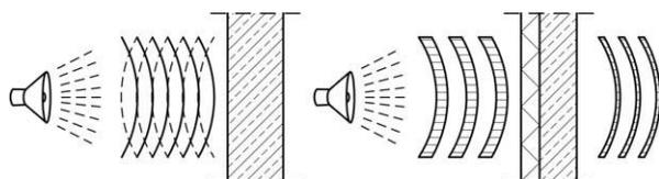
Figure 4: insulation - absorption [1]
